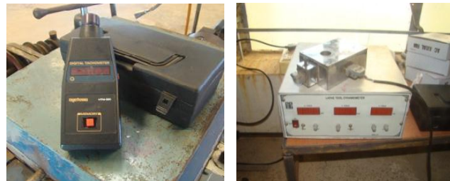
Fig 6 Tachometer and Lathe tool dynamometer
